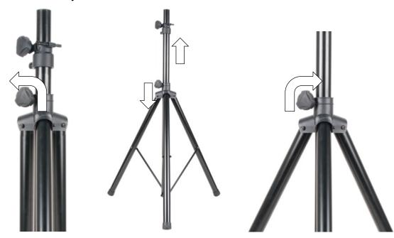
Loosen Knob A by turning it counter clockwise. Extend the inner pipe to the desired height and insert the safety pin through the stopper holes in the inner pipe. Secure and tighten Knob A by turning it clockwise.
